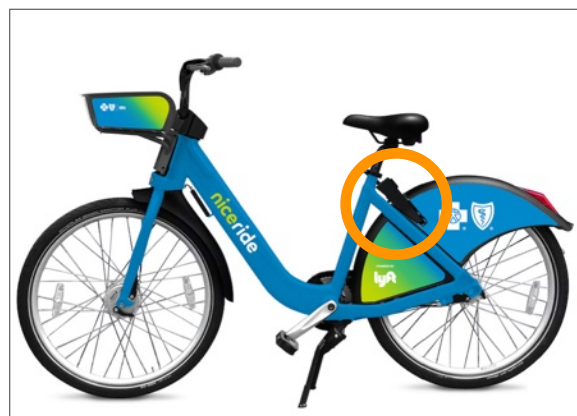
Figure 8: Dockless bike, with smart-lock shown in orange circle.
