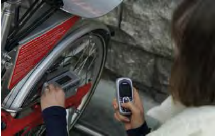
Figure 34 - User unlocking a Call a Bike with a combination code received by SMS
