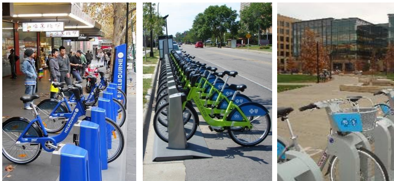
Figure 12 - Example Station Placements – Sidewalk (Melbourne Bike Share), In-Street (Nice Ride Minnesota), Public Plaza (Des Moines B-Cycle).
