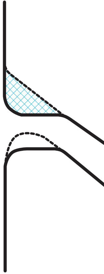
Converting an X-intersection into two Ts; Squaring off a Y-junction
