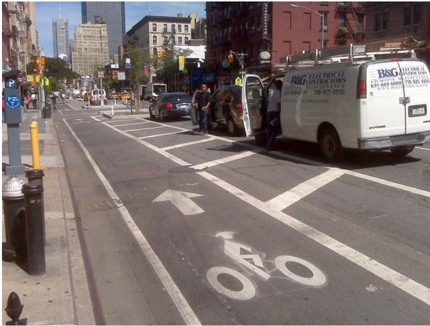
Figure 4-10: Sample Left-Side (and Traffic-Separated) Bike Lane, 9 th Avenue New York
