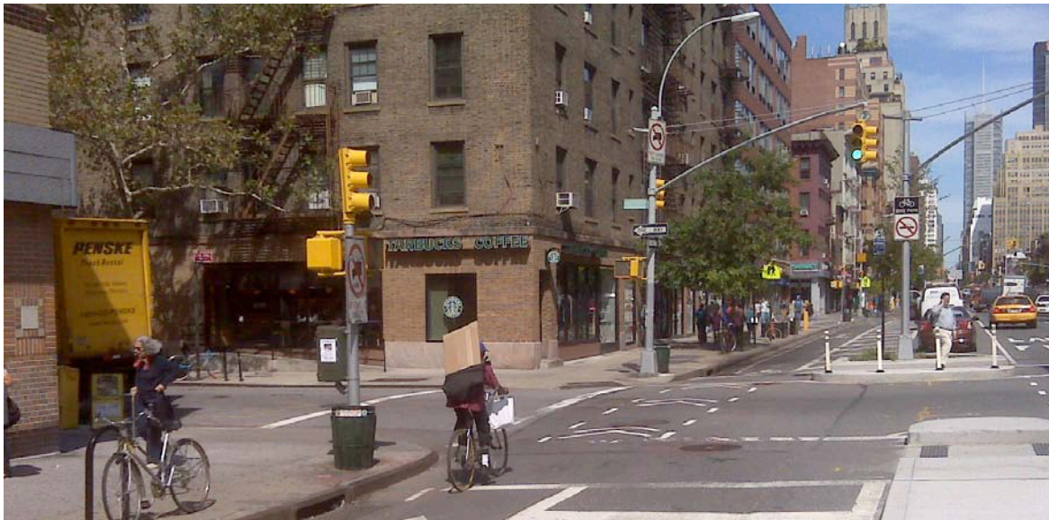
Figure 4-9: Sample Island-Separated Bike Lane, 9 th Avenue New York
